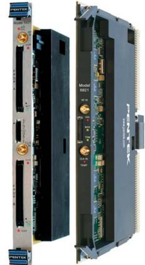
Model 6821 commercial (left) and conduction-cooled version
